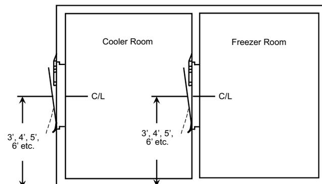
Note: The Partition Door Must Open Into The 35" Compartment.
